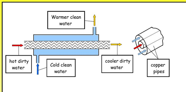
The diagram above shows a double pipe heat exchanger of the type used to improve energy efficiency in hospital laundry systems. Hot dirty water from the washing flows along the central pipe and clean cold water is passed through a cylindrical jacket surrounding the hot pipe. In this way, heat is transferred to the clean water which then requires less heating for use in the washing process.
