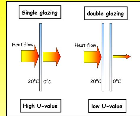
In a **cold** climate a building element with a **low U-value** will reduce **heat loss to the outside** and in a **hot** climate it will reduce **heat gain from outside**.
