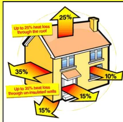
**Conduction** is the main thermal energy transfer process by which heat is lost from a building. The leakage of heat occurs through the walls, windows and roof and it can be reduced by the use of building materials which are **good thermal insulators**.
