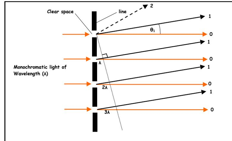
The above diagram shows a small section of a diffraction grating on which monochromatic light of wavelength ( $\lambda$ ) is normally incident. Consider what happens after the light passes through the grating.
