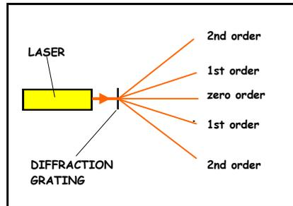
The diffraction images observed include the **ZERO ORDER** image which is along the straight-through position, with further images on either side which are referred to as the **1st ORDER**, **2nd ORDER** and so on.
