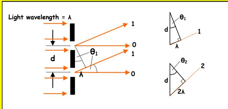
The light waves travelling along direction 1 interfere constructively to give the **1st ORDER MAXIMUM**. For this to happen, the PD for light waves from adjacent slits =  $1 \lambda$ .
