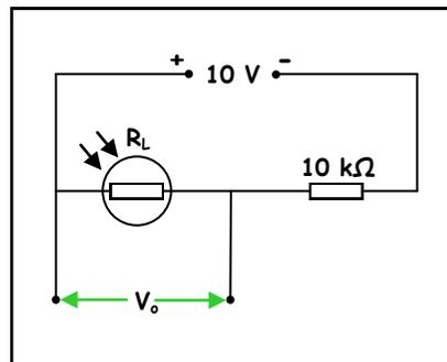
(b) The **value of  $R_L$**  in lighting conditions for which  $V_o = 4.0 \text{ V}$ .
