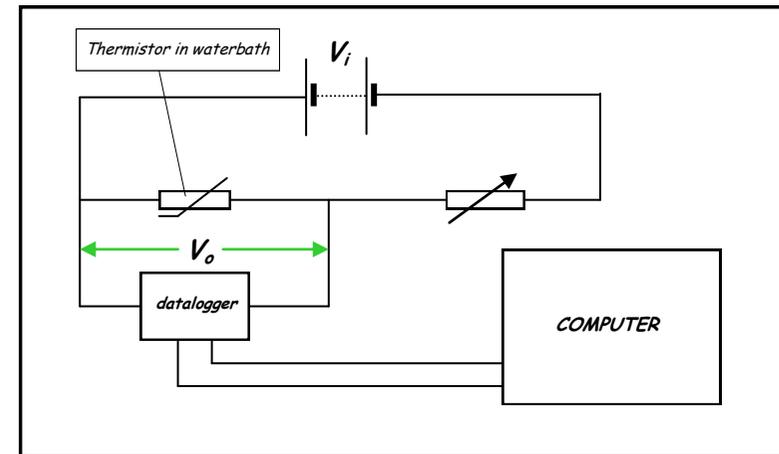
The circuit shown above may be used to investigate the variation of output pd ( $V_o$ ) with temperature for a **temperature-dependent potential divider**.
