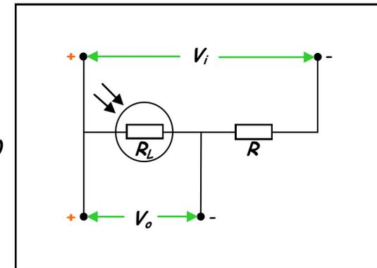
An LDR is a resistor made from semiconducting material in which electrons are liberated when light shines on the surface of the material.
