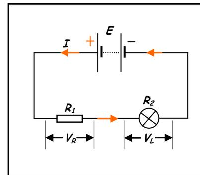
Energy supplied per coulomb by The battery (i.e. the e.m.f.) = The sum of the energies converted per coulomb in each component (i.e. the sum of the pd's)
