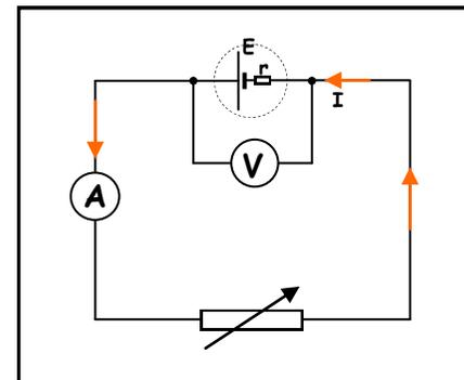
Corresponding values of the **current (I)** in the cell and **pd (V)** across the cell are obtained by adjusting the variable resistor. The results are recorded in the table shown below.
