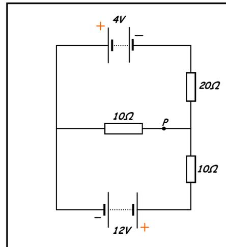
4 Use Kirhhoff's laws to determine the **current readings** shown on the ammeters ( $A_1$ ,  $A_2$  &  $A_3$ ) in the circuit shown opposite.
