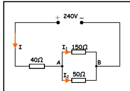
6 In the circuit shown opposite the voltmeter gives a reading of **8 V**. Calculate :
