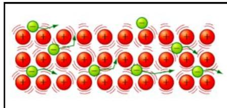
As a result, the electron-ion collisions are more frequent and this means that the flow of electrons is slowed down (i.e. the current is reduced).
