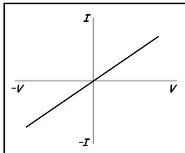
$$\text{Gradient of the } I\text{-}V \text{ graph} = 1/R.$$
