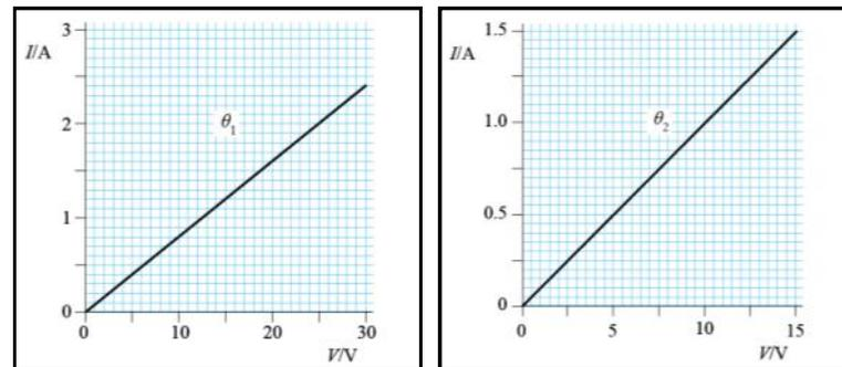
The above graphs show the I-V characteristics for a metal wire at two different temperatures  $\theta_1$  and  $\theta_2$ .
