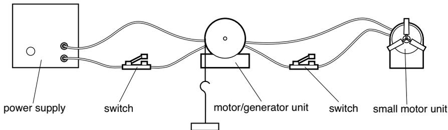
2. First, raise the mass by pressing the left-hand switch to connect the power supply to the motor/generator unit. *Gradually* increase the voltage until the mass starts to rise slowly.
