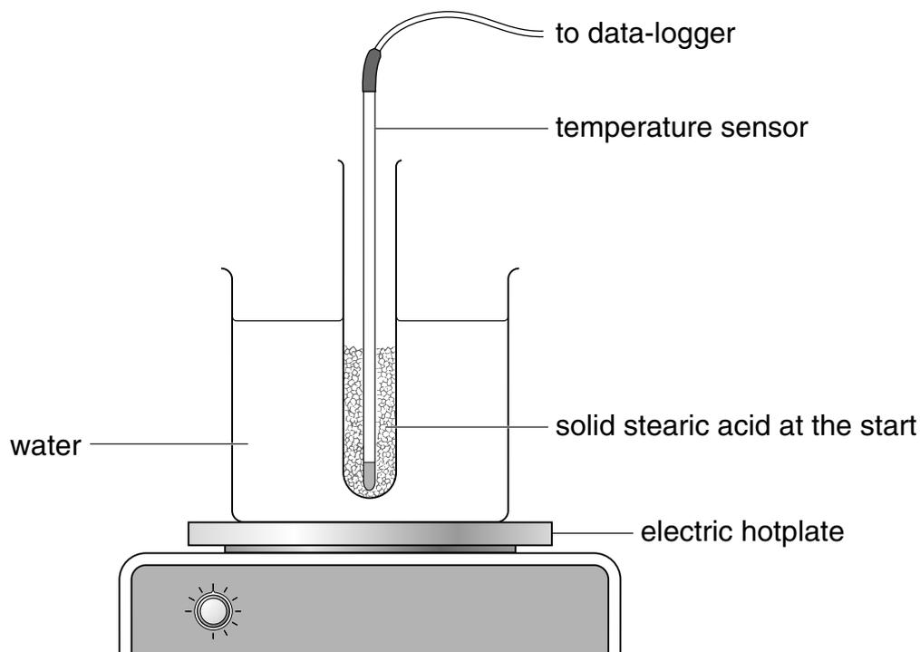
He used a temperature sensor attached to a data-logger to record the temperature of the stearic acid over a period of 35 minutes. A graph of the results is shown below.
