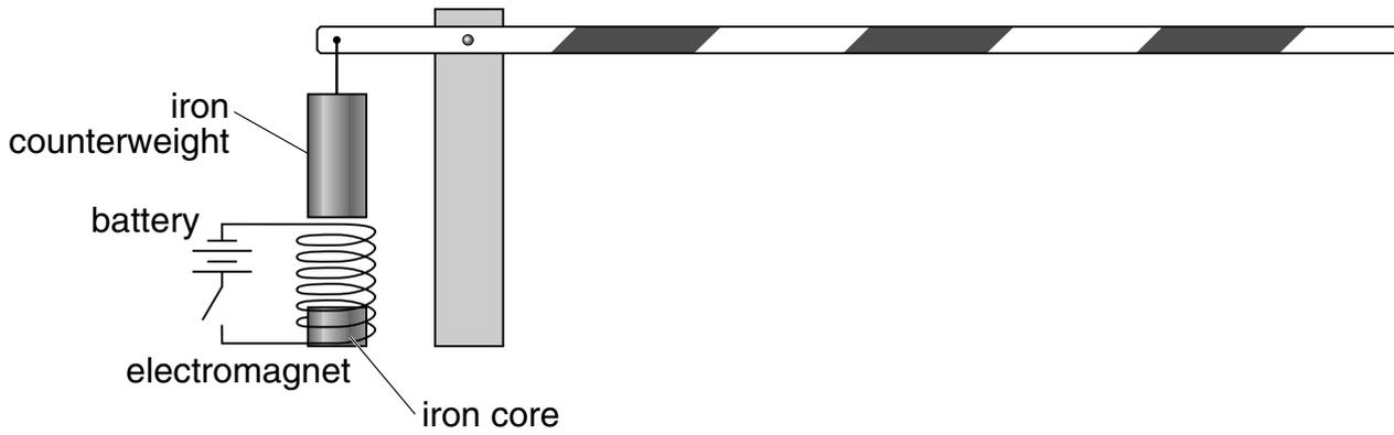
When the switch is closed the barrier rises.
