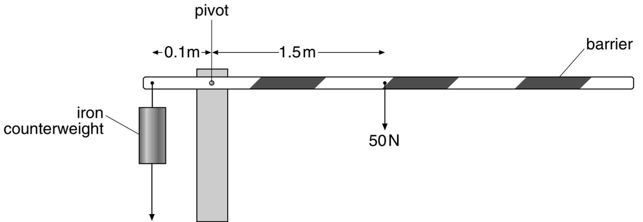
(i) Calculate the turning moment produced by the barrier about the pivot.
